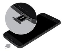
3. Slide the SIM card/Memory card tray back into the slot.
